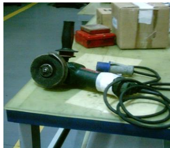
Water entered from the grinding machine vent point
