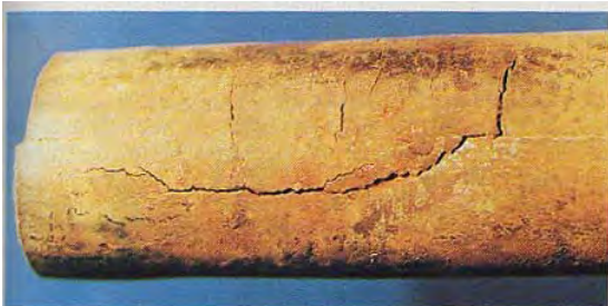
Both longitudinal and transverse stress-corrosion cracks on a brass heat exchanger tube that had been exposed to ammonia. Note the branching of the cracks.
