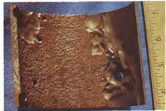
Smooth attack on carbon steel by carbonic acid. Note the vivid red color of hematite, indicating high oxygen concentrations.
