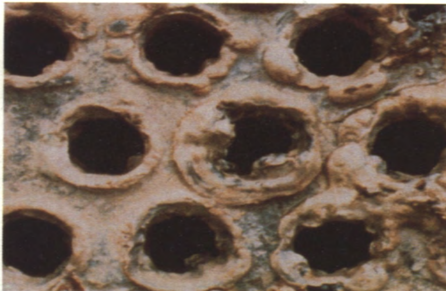
Fouling reduces exchanger's heat transfer efficiency.
