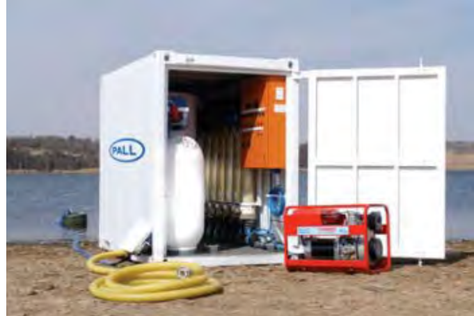
Figure 4b. Small flow Container Up to 1200 m 3 /d
