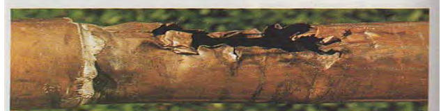
A large, ragged perforation in a region of severe internal wastage on a copper pipe. Corrosion was caused by ammonia-containing condensate.
