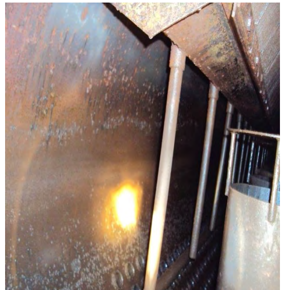
Figure 2: pitting corrosion inside steam drum of an O-type Boiler
