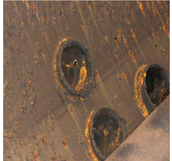
Figure 1: pitting corrosion inside steam drum of an O-type Boiler
