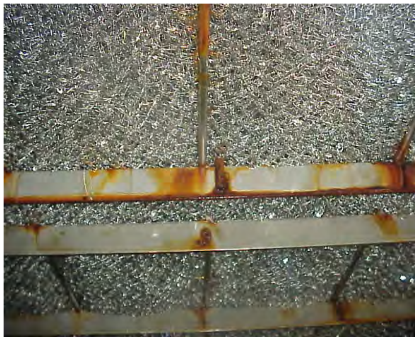
Figure (6).Clean demister. (After Acid Clean ).
