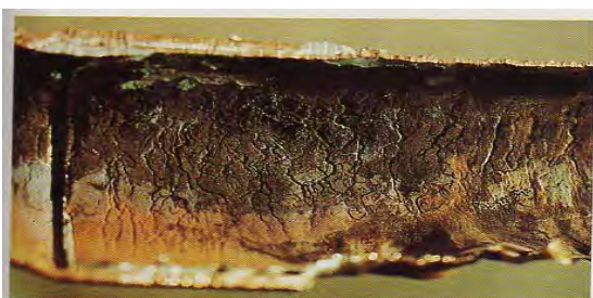
Severe grooving on the internal surface of a copper pipe carrying condensate. Grooves were cut by condensing vapors running down pipe walls. Note the vivid blue corrosion products and deposits near the bottom.
