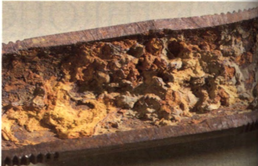
Deposition of corrosion products and scales in Cooling systems which restrict the water flow and also leading to tube failure .
