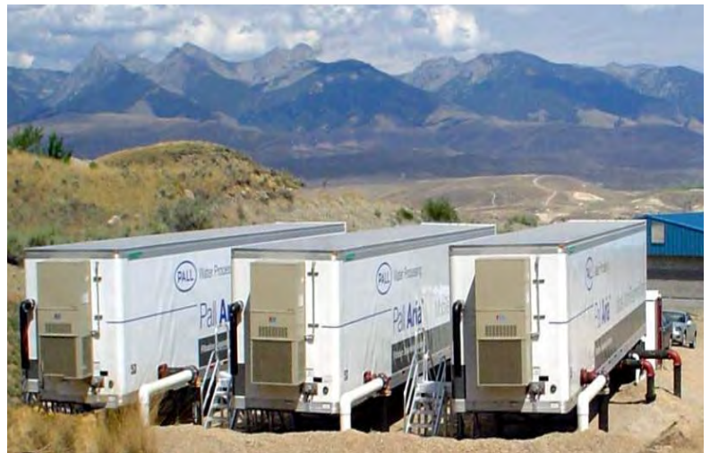
Fig15: Membranes containerized mobile systems
