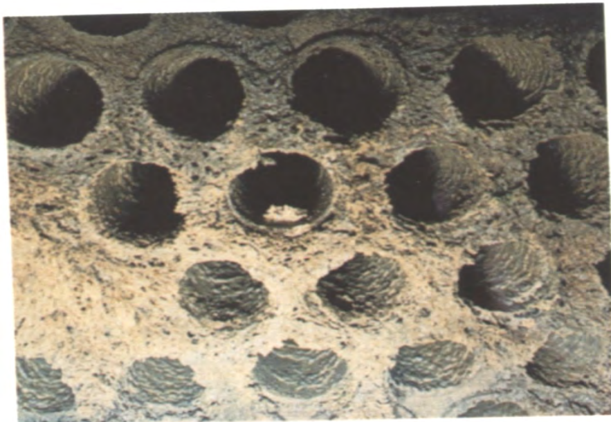
Calcium carbonate scaling of an electric utility surface condenser due to poor treatment
